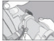
Step #3: Insert strainer or fitting into quick connect port, push all the way until stops.
