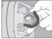
Step #2: Using your thumb, pry up edge of lock clip over lock tab. (as shown)
