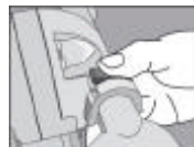
Step #5: Snap lock clip over fitting and lock. Pull fitting to make sure is locked in. to place.
